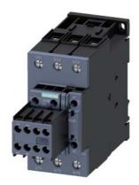
power contactor, AC-3e/AC-3, 80 A, 37 kW / 400 V, 3-pole, 110 V AC, 50/60 Hz, auxiliary contacts: 2 NO + 2 NC, screw terminal, size: S2, removable auxiliary switch
