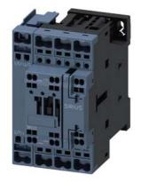
contactor AC-1, 50 A, 400 V / 40 °C, 4-pole, 24 V AC, 50/60 Hz, auxiliary contacts: 1 NO + 1 NC, spring-loaded terminal, size: S0
