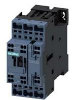
power contactor, AC-3e/AC-3, 17 A, 7.5 kW / 400 V, 3-pole, 200-280 V AC/DC, 50/60 Hz, with integrated varistor, auxiliary contacts: 1 NO + 1 NC, spring-loaded terminal, size: S0
