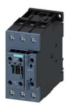
power contactor, AC-3e/AC-3, 65 A, 30 kW / 400 V, 3-pole, 20-33 V AC/DC, 50/60 Hz, with integrated varistor, auxiliary contacts: 1 NO + 1 NC, screw terminal, size: S2, communication-capable
