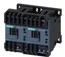
reversing contactor assembly, AC-3e/AC-3, 12 A, 5.5 kW / 400 V, 3-pole, 230 V AC, 50/60 Hz, spring-loaded terminal, electrical and mechanical interlock
