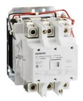
Mechanically held lighting contactor, Contactor amp rating 200A, 0 N.C. / 5 N.O. poles, 110VAC 50HZ/120VAC 60HZ coil, Non-combination type, Enclosure NEMA type (open), No enclosure
