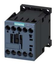
power contactor, AC-3e/AC-3, 16 A, 7.5 kW / 400 V, 3-pole, 24 V DC, auxiliary contacts: 1 NC, screw terminal, size: S00, communication-capable
