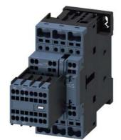
power contactor, AC-3e/AC-3, 38 A, 18.5 kW / 400 V, 3-pole, 230 V AC, 50/60 Hz, auxiliary contacts: 2 NO + 2 NC, spring-loaded terminal, size: S0, removable auxiliary switch
