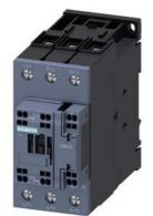
power contactor, AC-3e/AC-3, 51 A, 22 kW / 400 V, 3-pole, 110 V AC, 50/60 Hz, auxiliary contacts: 1 NO + 1 NC, main circuit: screw terminal, control and auxiliary circuit: spring-loaded terminal, size: S2
