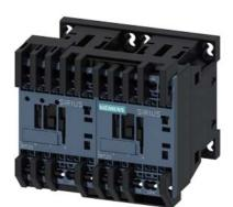
reversing contactor assembly, AC-3e/AC-3, 7 A, 3 kW / 400 V, 3-pole, 24 V DC, spring-loaded terminal, electrical and mechanical interlock, with voltage tap for 3RA27
