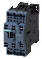
traction contactor, AC-3e/AC-3, 17 A, 7.5 kW / 400 V, 3-pole, 24 V DC, 0.7-1.25  $^{\star}$  Us, electronic drive, with integrated varistor, auxiliary contacts: 1 NO + 1 NC, spring-loaded terminal, size: S0
