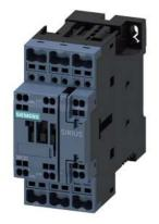
traction contactor, AC-3e/AC-3, 32 A, 15 kW / 400 V, 3-pole, 72 V DC, 0.7-1.25\* Us, electronic drive, with integrated varistor, auxiliary contacts: 1 NO + 1 NC, spring-loaded terminal, size: S0
