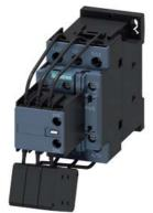
capacitor contactor, AC-6b 20 kVAr, / 400 V, 3-pole, 230 V AC, 50 Hz, auxiliary contacts: 1 NO + 2 NC, screw terminal, size: S0
