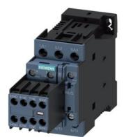
power contactor, AC-3e/AC-3, 17 A, 7.5 kW / 400 V, 3-pole, 24 V DC, with plugged-in diode combination, auxiliary contacts: 3 NO + 3 NC, screw terminal, size: S0, with 3RH2911-1XA22-0MA0
