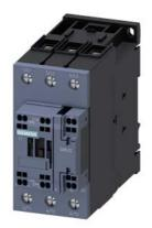
power contactor, AC-3e/AC-3, 41 A, 18.5 kW / 400 V, 3-pole, 220 V AC, 50/60 Hz, auxiliary contacts: 1 NO + 1 NC, main circuit: screw terminal, control and auxiliary circuit: spring-loaded terminal, size: S2
