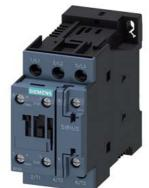
power contactor, AC-3e/AC-3, 38 A, 18.5 kW / 400 V, 3-pole, 110 V DC, auxiliary contacts: 1 NO + 1 NC, screw terminal, size: S0
