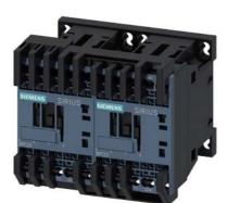
reversing contactor assembly, AC-3e/AC-3, 12 A, 5.5 kW / 400 V, 3-pole, 24 V AC, 50/60 Hz, spring-loaded terminal, electrical and mechanical interlock
