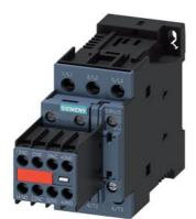
power contactor, AC-3e/AC-3, 12 A, 5.5 kW / 400 V, 3-pole, 24 V DC, with plugged-in varistor, auxiliary contacts: 2 NO + 2 NC, screw terminal, size: S0, captive auxiliary switch
