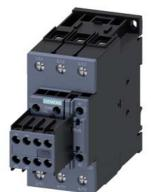
power contactor, AC-3e/AC-3, 65 A, 30 kW / 400 V, 3-pole, 220 V AC, 50/60 Hz, auxiliary contacts: 2 NO + 2 NC, screw terminal, size: S2, removable auxiliary switch
