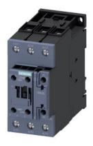
power contactor, AC-3e/AC-3, 51 A, 22 kW / 400 V, 3-pole, 24 V DC, 0.8-1.2\* Us, with integrated varistor, auxiliary contacts: 1 NO + 1 NC, screw terminal, size: S2, suitable for PLC outputs, upright mounting position
