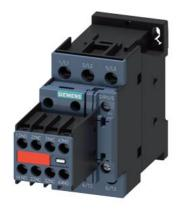
power contactor, AC-3e/AC-3, 38 A, 18.5 kW / 400 V, 3-pole, 110 V AC, 50 Hz / 120 V, 60 Hz, auxiliary contacts: 2 NO + 2 NC, screw terminal, size: S0, captive auxiliary switch, no surge suppressor retrofittable
