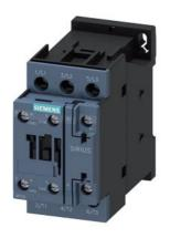
contactor, NEMA version, 10 hp, 460 / 575 V, 3-pole, 240 V AC, 50/60 Hz, auxiliary contacts: 1 NO + 1 NC, screw terminal, size: S0  $\,$
