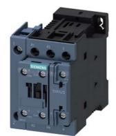
traction contactor, AC-3, 25 A, 11 kW / 400 V, 4-pole, 24 V DC, 0.7-1.25\* Us, electronic drive, with integrated varistor, main contacts: 2 NO + 2 NC, auxiliary contacts: 1 NO + 1 NC, screw terminal, size: S0
