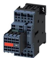
power contactor, AC-3e/AC-3, 25 A, 11 kW / 400 V, 3-pole, 230 V AC, 50/60 Hz, auxiliary contacts: 2 NO + 2 NC, spring-loaded terminal, size: S0, captive auxiliary switch, no surge suppressor retrofittable
