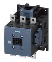
power contactor, AC-3e/AC-3 300 A, 160 kW / 400 V, AC (50-60 Hz) / DC Uc: 220-240 V 3-pole, auxiliary contacts 2 NO + 2 NC drive: conventional main circuit: busbar control and auxiliary circuit: screw terminal
