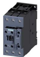
power contactor, AC-3e/AC-3, 51 A, 22 kW / 400 V, 3-pole, 600 V AC, 60 Hz, auxiliary contacts: 1 NO + 1 NC, screw terminal, size: S2  $\,$
