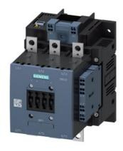
power contactor, AC-3e/AC-3 185 A, 90 kW / 400 V Uc: 24 V DC x (0.7-1.25) PLC input 24-110 V DC 3-pole, auxiliary contacts 2 NO + 2 NC drive: electronic main circuit: busbar control and auxiliary circuit: spring-loaded terminal extended rated condition railroad IEC 60077
