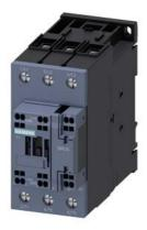
power contactor, AC-3e/AC-3, 41 A, 18.5 kW / 400 V, 3-pole, 48 V AC, 50 Hz, auxiliary contacts: 1 NO + 1 NC, main circuit: screw terminal, control and auxiliary circuit: spring-loaded terminal, size: S2
