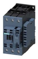
power contactor, AC-3e/AC-3, 41 A, 18.5 kW / 400 V, 3-pole, 230 V AC, 50 Hz, auxiliary contacts: 2 NO + 2 NC, main circuit: screw terminal, control and auxiliary circuit: spring-loaded terminal, size: S2, lateral auxiliary switch
