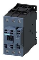
traction contactor, AC-3e/AC-3, 51 A, 22 kW / 400 V, 3-pole, 72 V DC, 0.7-1.25\* Us, electronic drive, with integrated varistor, auxiliary contacts: 1 NO + 1 NC, main circuit: screw terminal, control and auxiliary circuit: spring-loaded terminal, size: S2
