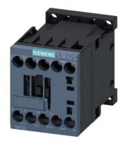
power contactor, AC-3e/AC-3, 9 A, 4 kW / 400 V, 3-pole, 24 V AC, 50/60 Hz, auxiliary contacts: 1 NO, screw terminal, size: S00, upright mounting position
