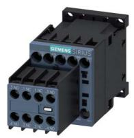
power contactor, AC-3e/AC-3, 16 A, 7.5 kW / 400 V, 3-pole, 24 V DC, with integrated diode, auxiliary contacts: 3 NO + 2 NC, screw terminal, size: S00, removable auxiliary switch
