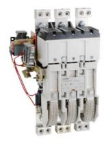
Mechanically held lighting contactor, Contactor amp rating 400A, 0 N.C. / 3 N.O. poles, 220VAC 50HZ/240VAC 60HZ coil, Non-combination type, Enclosure NEMA type (open), No enclosure
