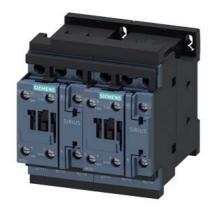
reversing contactor assembly, AC-3e/AC-3, 12 A, 5.5 kW / 400 V, 3-pole, 230 V AC, 50/60 Hz, screw terminal, electrical and mechanical interlock, auxiliary contacts: 2 x 1 NO
