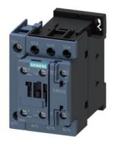
contactor AC-1, 50 A, 400 V / 40 °C, 4-pole, 230 V AC, 50 Hz, auxiliary contacts: 1 NO + 1 NC, screw terminal, size: S0
