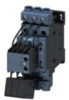
capacitor contactor, AC-6b 33 kVAr, / 400 V, 3-pole, 24 V AC, 50/60 Hz, auxiliary contacts: 1 NO + 2 NC, screw terminal, size: S0
