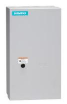
Mechanically held lighting contactor, Contactor amp rating 200A, 0 N.C. / 4 N.O. poles, 440VAC 50HZ/480VAC 60HZ coil, Non-combination type, Enclosure NEMA type 1, Indoor general purpose use
