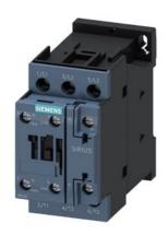
power contactor, AC-3e/AC-3, 25 A, 11 kW / 400 V, 3-pole, 208 V AC, 50/60 Hz, auxiliary contacts: 1 NO + 1 NC, screw terminal, size: S0, upright mounting position
