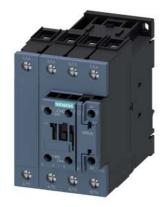
contactor AC-1, 60 A, 400 V / 40 °C, 4-pole, 230 V AC, 50 Hz, auxiliary contacts: 1 NO + 1 NC, screw terminal, size: S2
