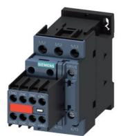
power contactor, AC-3e/AC-3, 25 A, 11 kW / 400 V, 3-pole, 110 V AC, 50 Hz / 120 V, 60 Hz, auxiliary contacts: 2 NO + 2 NC, screw terminal, size: S0, captive auxiliary switch, no surge suppressor retrofittable
