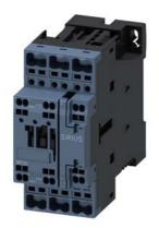
power contactor, AC-3e/AC-3, 12 A, 5.5 kW / 400 V, 3-pole, 24 V DC, auxiliary contacts: 1 NO + 1 NC, spring-loaded terminal, size: S0, communication-capable
