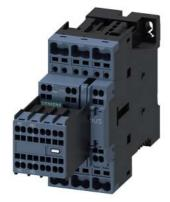
power contactor, AC-3e/AC-3, 17 A, 7.5 kW / 400 V, 3-pole, 24 V DC, auxiliary contacts: 2 NO + 2 NC, spring-loaded terminal, size: S0, removable auxiliary switch
