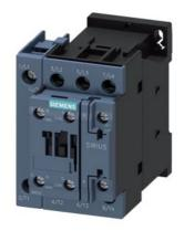
contactor AC-1, 40 A, 400 V / 40  $^{\circ}$ C, 4-pole, 480 V AC, 60 Hz, auxiliary contacts: 1 NO + 1 NC, screw terminal, size: S0
