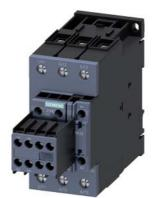
power contactor, AC-3e/AC-3, 80 A, 37 kW / 400 V, 3-pole, 220 V AC, 50/60 Hz, auxiliary contacts: 2 NO + 2 NC, screw terminal, size: S2, removable auxiliary switch
