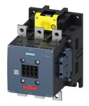
power contactor, AC-3e/AC-3 225 A, 110 kW / 400 V AC (50-60 Hz) / DC 200-277 V x (0.8-1.1) F-PLC input 24 V DC 3-pole, auxiliary contacts 2 NO + 2 NC permanently mounted drive: electronic main circuit: busbar control and auxiliary circuit: screw terminal
