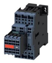
power contactor, AC-3e/AC-3, 25 A, 11 kW / 400 V, 3-pole, 24 V DC, auxiliary contacts: 2 NO + 2 NC, spring-loaded terminal, size: S0, captive auxiliary switch, no surge suppressor retrofittable
