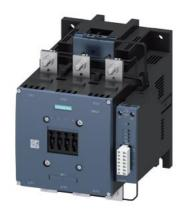
power contactor AC-1 690 A / 690 V / 40  $^{\circ}$ C 3-pole, Uc: 96-127 V AC(50-60 Hz) / DC PLC input 24 V DC drive: electronic auxiliary contacts 2 NO + 2 NC main circuit: busbar control and auxiliary circuit: screw terminal with remaining lifetime indicator
