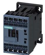
power contactor, AC-3e/AC-3, 12 A, 5.5 kW / 400 V, 3-pole, 24 V DC, auxiliary contacts: 1 NC, spring-loaded terminal, size: S00, upright mounting position
