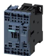
contactor AC-1, 35 A, 400 V / 40 °C, 4-pole, 220 V DC, auxiliary contacts: 1 NO + 1 NC, spring-loaded terminal, size: S0
