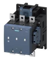
vacuum contactor AC-3e/AC-3 300 A, 160 kW / 400 V, 3-pole, Uc: 220-240 V AC(50-60 Hz) / DC drive: conventional auxiliary contacts 2 NO + 2 NC main circuit: busbar control and auxiliary circuit: screw terminal
